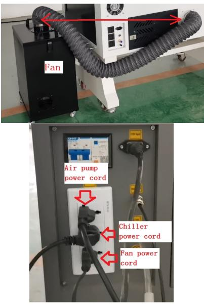
Note: If the machine is powered by AC110V, the socket on the machine is also 110V, so be sure to check the power supply voltage level of the chiller, fan, and air pump. The voltage levels of these three are required to be consistent with the machine voltage levels. In other words, if the voltage level on the label on the back of the machine is 220V, the power supply voltage of the chiller, air pump and fan should also be 220V
