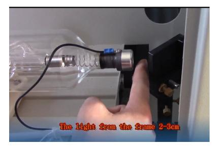
(7) Finally, fix the laser tube, fix the bracket, and complete the installation.
