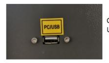
Connect the PC/USB interface of the machine to the USB interface of the computer with a data cable
