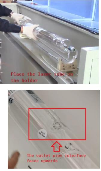
(2) Install the laser tube inlet pipe, as shown in the figure below:
